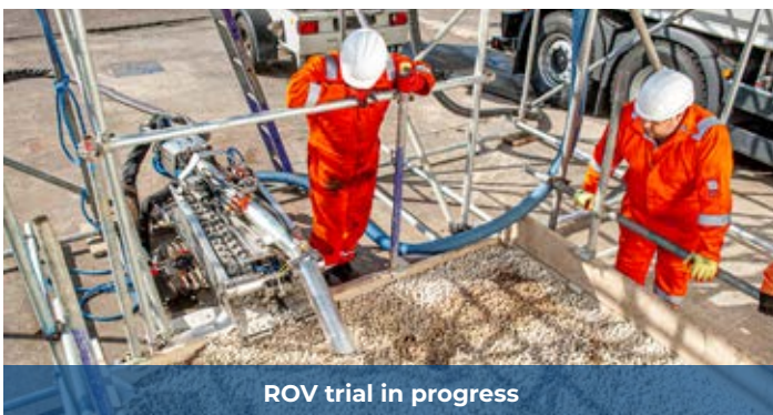
Demonstration of scaffold set up, aggregate and ROV being lowered
